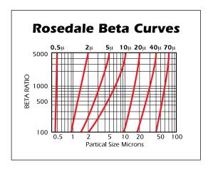
The Beta Ratio (ß) at a given particle size can be correlated to the filter efficiency at that particle size according to the following formula:
